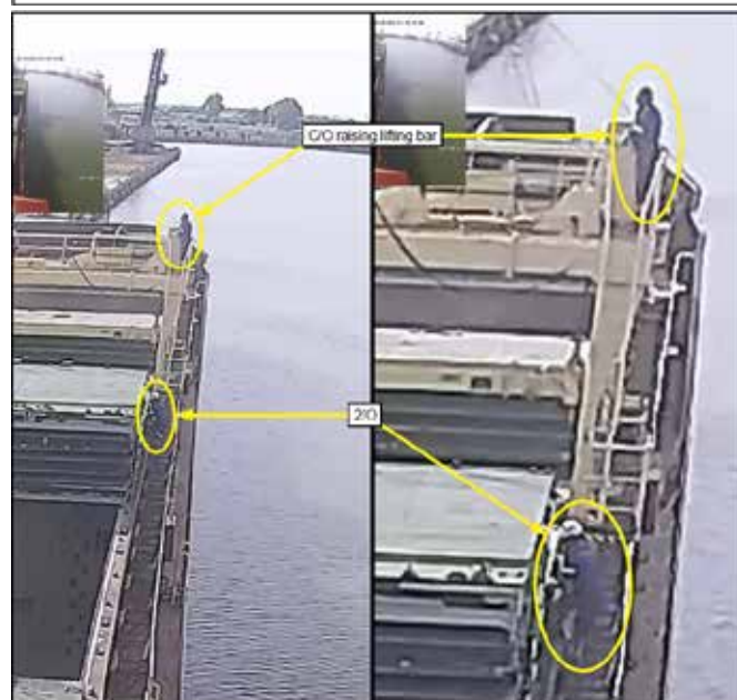
Zoomed CCTV screenshot showing the 2nd Officer climbing onto cargo hold hatch coaming
