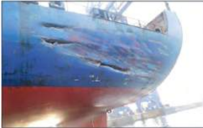
Damage to the container port quarter
