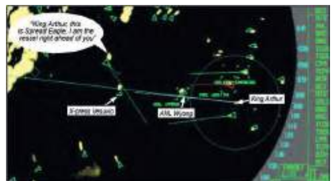
Detail of the gas carrier radar when called by another approaching target showing that, there were three vessels that could be assessed as 'ahead' of the gas carrier
