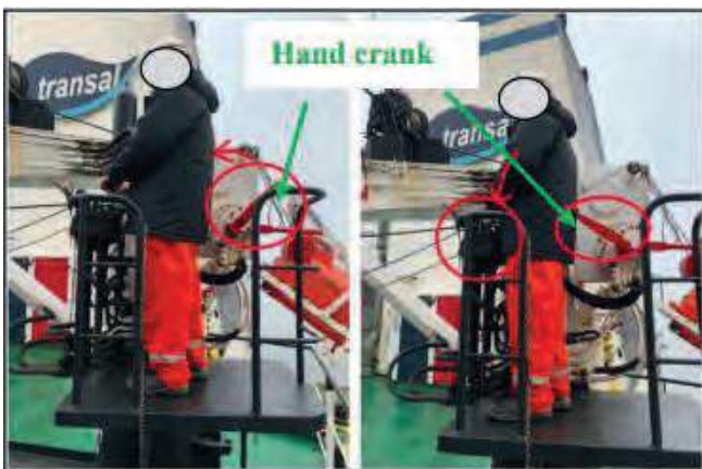
A simulation of the bosun's position while handling the control box, with his back to the hand crank
