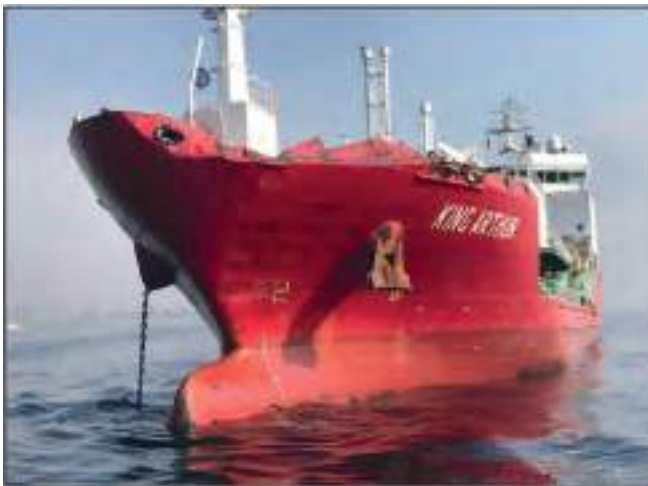
Damage to the gas carrier port bow
