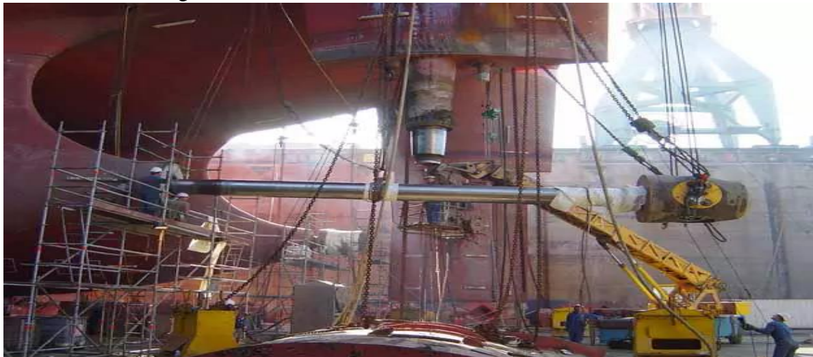
Figure 77: Propeller shaft withdrawal (Diesel Ship, 2017)
